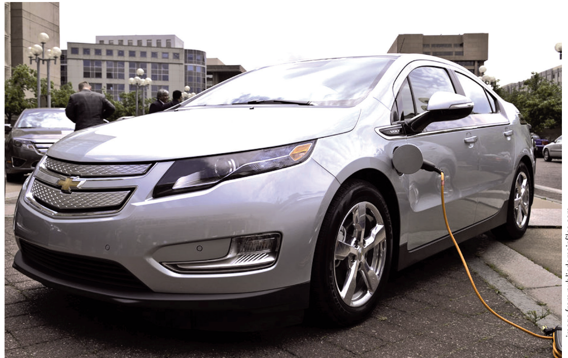
Pictured above is a Chevy Volt, an electric hybrid car (shown here plugged in). This car operates as a pure battery vehicle with a gas powered internal combustion engine to extend the car's range as needed.
